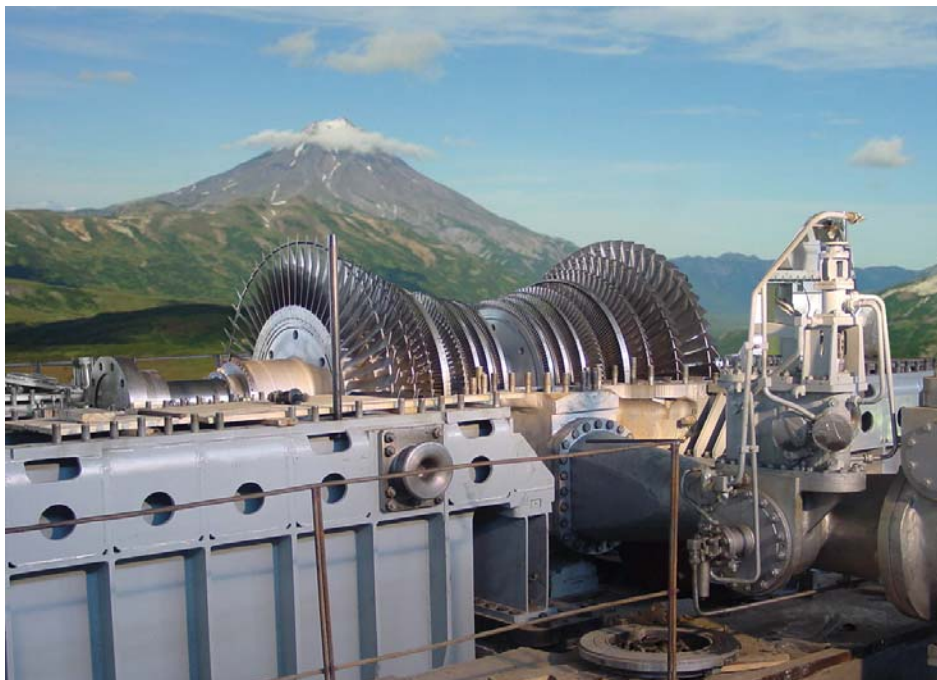
Fig. 10. 25 MW steam turbine worked out and manufactured by “KTZ” SC for Mutnovsky GeoPP.
