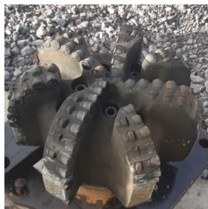
Figure 5: PDC Bit Ring out on the shoulder
