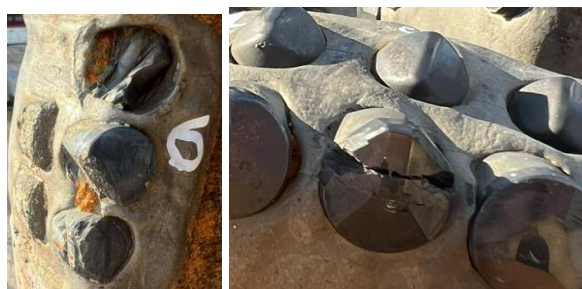
Figure 3: Picture of Broken Cutters. Front faced overload (left) and tangential diamond table fracture (right)
