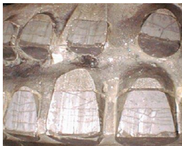
Figure 8: Stick slip vibration heat checking located on the tungsten carbide substrate
