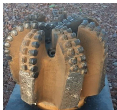
Figure 1: Picture of used PDC drill bit used in a Contact Energy, New Zealand Geothermal Application
