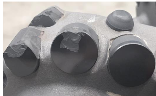
Figure 4: Picture of chipped cutters exhibiting thermal degradation.
