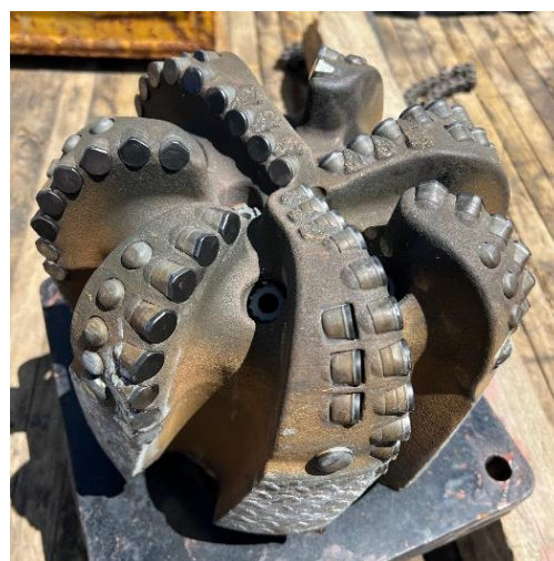
Figure 9: 12" PDC Bit Dull in Geothermal Application, NZ
