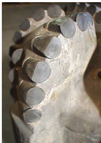
Figure 7: Worn Teeth even wear flats across all cutters. No indication of thermal wear indicates only abrasive wear mode. This is considered a normal dull mechanism.
