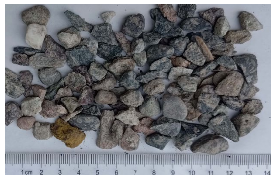
Photo 2: A photo of the silica sand filled in the GHE.
