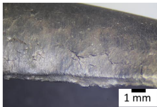
(a) Cracks branching from the score line.
