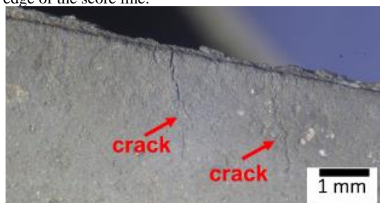
(b) Cracks propagated from the edge of the score line.
