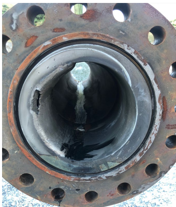
Figure 6: Straight Thru pipe erosion - end view.
