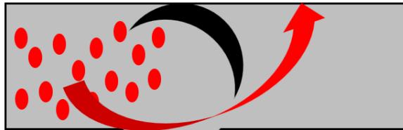
Figure 9: Steam flow direction during partial valve opening.
