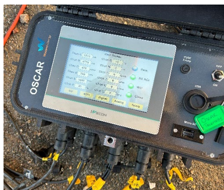
Figure 13: 'Oscar' telemetry unit for data gathering and transmission.
