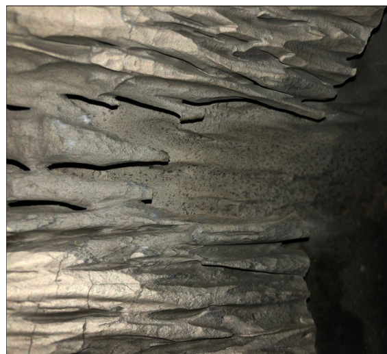
Figure 7: Stellite hard facing eroded by high velocity steam and cuttings.
