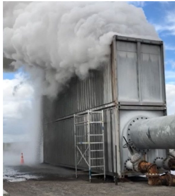
Figure 10: Brine carryover from the base model LECM while exceeding design capacity.
