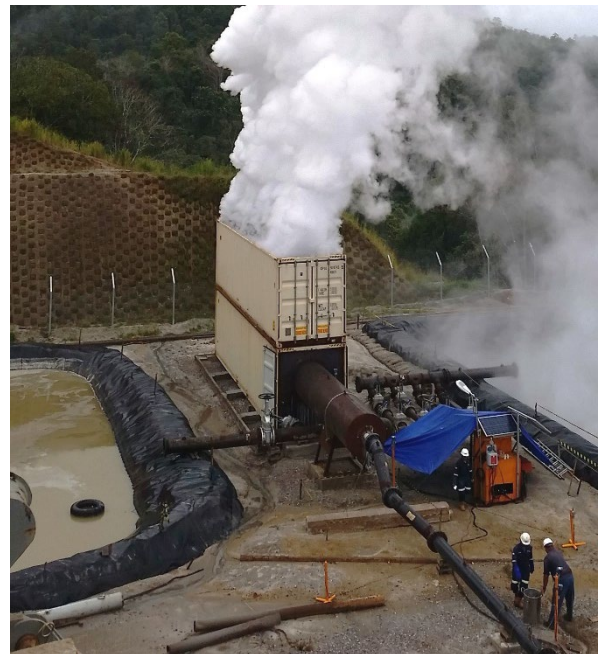
Figure 11: LECM base model in Indonesia at design capacity with no carryover.
