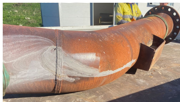
Figure 3: S-Bend with pinhole failure.
