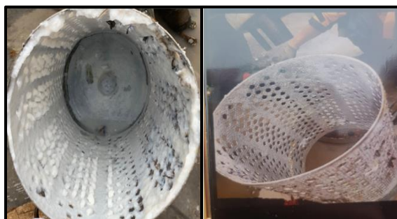
Figure 5: Left side: strainer brine pump B without chemical treatment. Right side: Strainer brine pump B with 10ppm chemical treatment.
