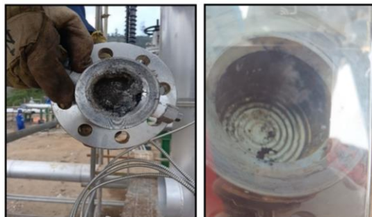
Figure 2: Comparison of level sensor before (left) and after (right) achieving the correct dosage.
