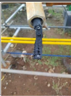
Figure 3: The coupon is a carbon steel C1018 type with 14 days of insertion. Scale was also obtained and analyzed using SEM/XRF.
