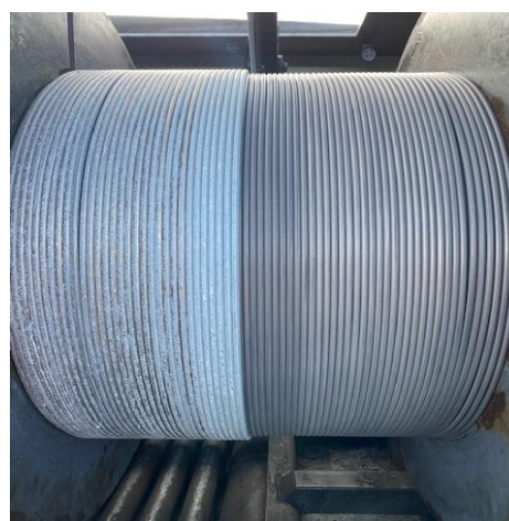
Figure 11: Example of the blue/white scale that previously formed on our downhole capillary tubing when overdosing the calcite inhibition chemical.
