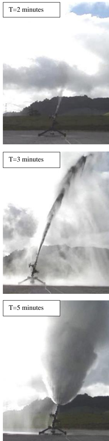
Figure 6 Vertical discharge sequence. See Figure 3 for timing – 6A T=2 minutes, gas-only discharge; 6B T=3 minutes, non-boiling liquid discharge; 6C T=5 minutes, Maximum two-phase flow
