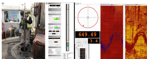
Figure 2: Acoustic borehole image acquisition. A) ABI43 tool pulled out of the well after logging. B) Screen during acquisition showing un-processed images while logging at well at location #3. Observations during logging provide first indications of borehole shape and potential fracture occurrence, though fractures are not necessarily permeable (see Section 3.2).
