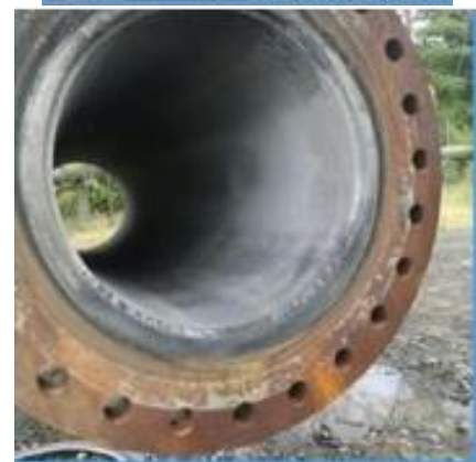
Figure 5: Pipeline inspection after the trial with Geogard®SX.
