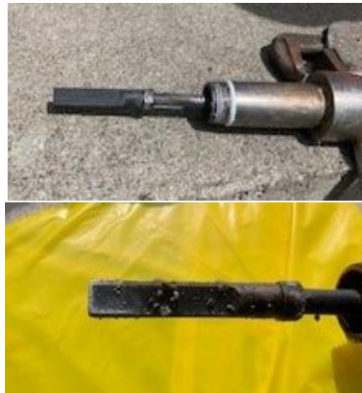
Figure 4: Point 2 coupons after the trial with Geogard®SX.
