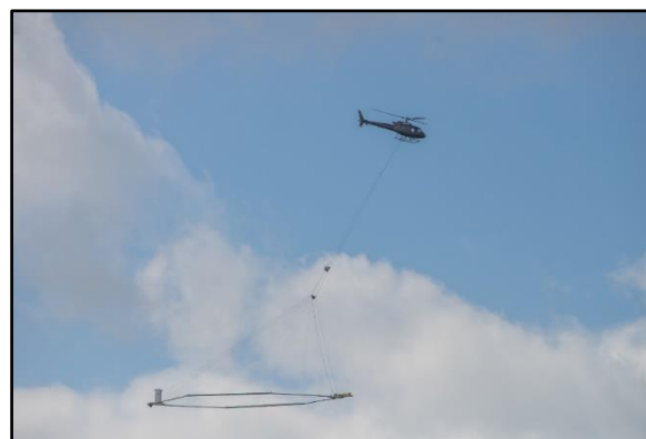
Figure 1: Typical SkyTEM configuration. The large loop below the helicopter contains both the transmitter and receiver loops. Photograph from SkyTEM.
