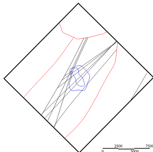
Figure 3: Plan view of updated fault network shown at -2800 masl (metres above sea level) in the model. This is taken from the Leapfrog digital conceptual model.
