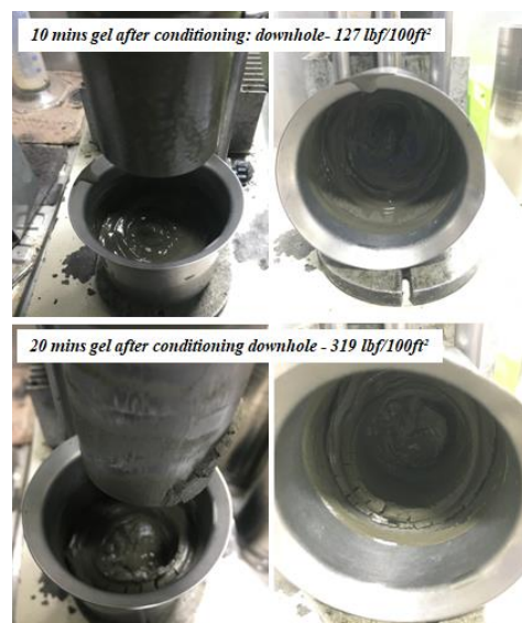
Figure 2 Pseudo Thixo Cement Slurry - Laboratory Test pictures after 10min and after 20min
