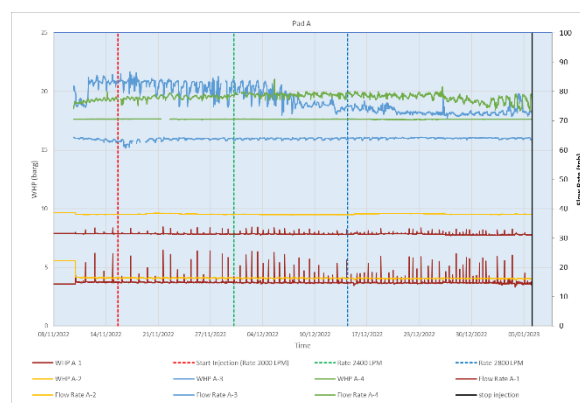
Figure 7: Relatively stable flow rate and well head pressure profile for Pad A wells during injection.
