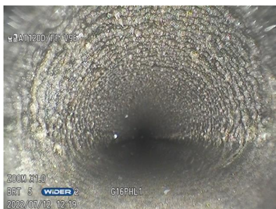
Figure 6 - Image of scaling within a G16 pre-heater tube
