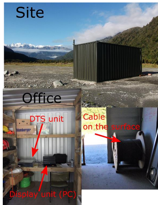
Figure 1: DFDP-2 drillsite. The site office is located in the shipping container placed over the borehole (wellhead is accessible through a cellar under the container floor). The measuring equipment, as well as the surface part of the cable, are placed inside the container.
