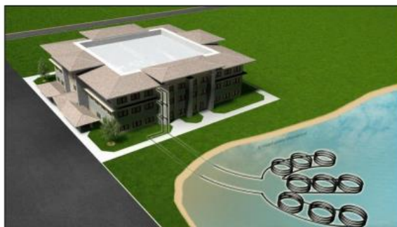
Figure 2: Open loop using a body of water such as a lake
