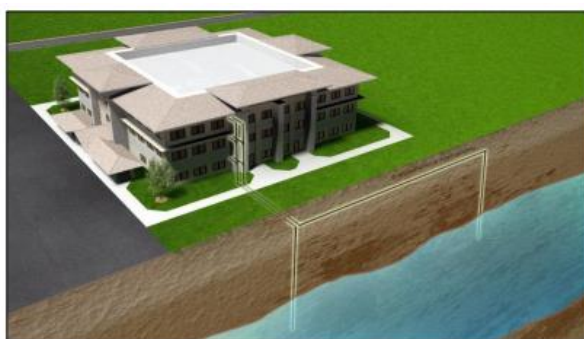
Figure 3: Paired boreholes to a nominal depth of 50m
