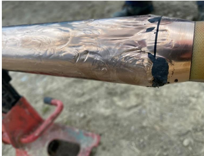
Figure 7: Erosion patterns on the BeCu25 downhole antenna
