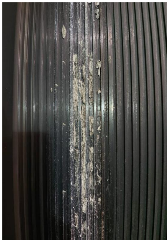
Figure 7: Mineral Deposits in Rotor Seal Grooves - Close View.
