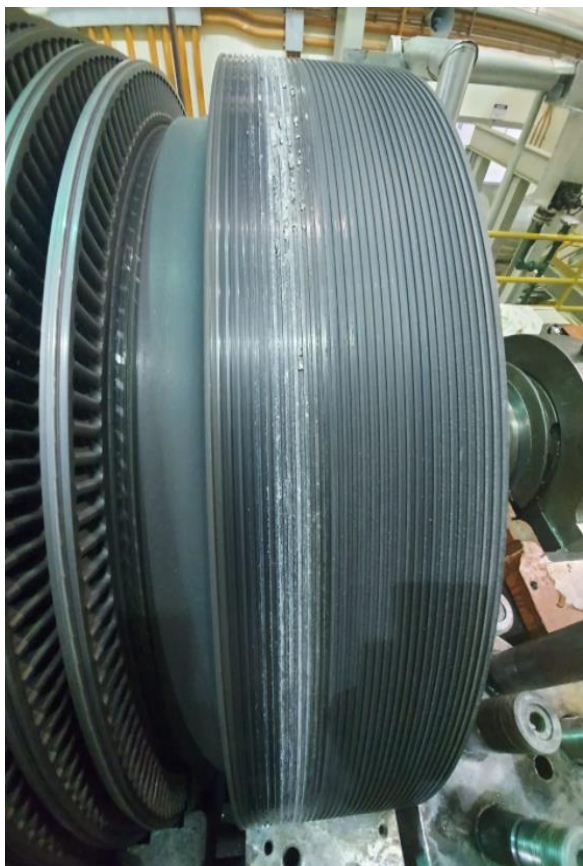
Figure 6: Mineral Deposits in Rotor Seal Grooves - Overall View
