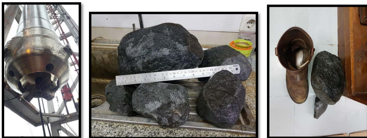
Figure 1: Worn out or ring out drill shoe and unconsolidated Andesitic Lava Sample that was caught by Fishing Tools
