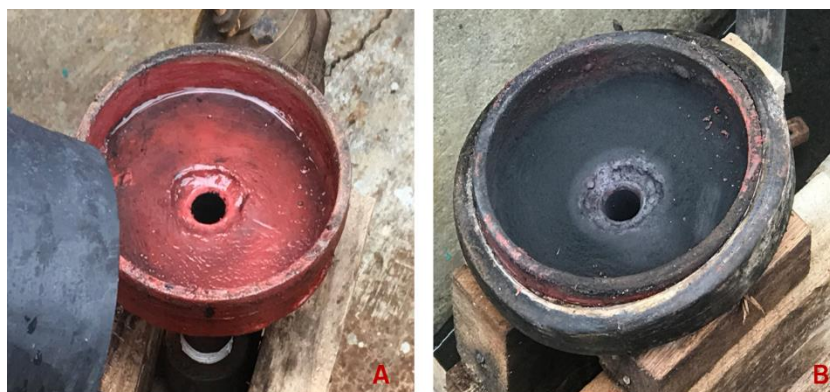
Figure 9. Scaling in the pipe holder for the dosed (A) and undosed (B) lines.
