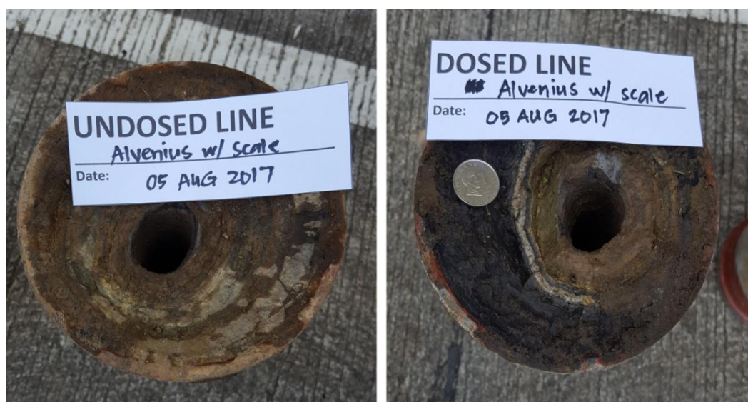
Figure 4. Pre-trial state of the dosed and undosed alvenius pipes
