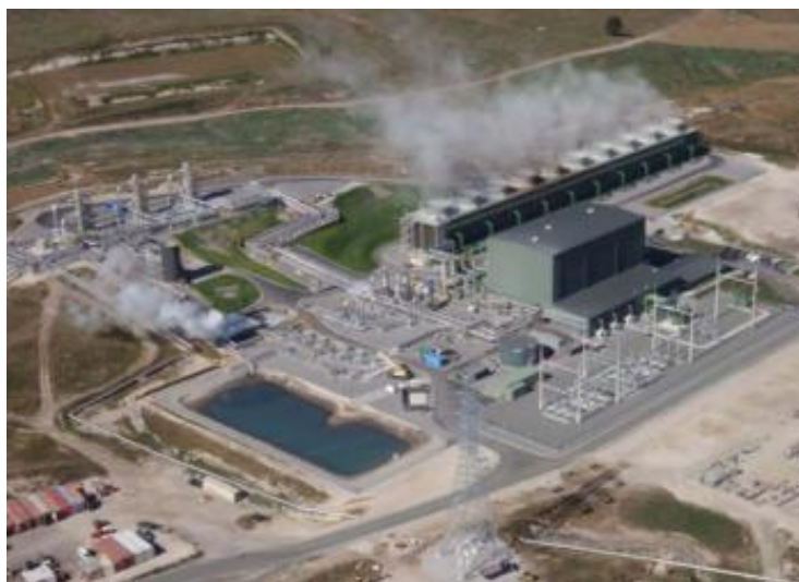
Figure 2. An aerial photo of the Nga Awa Purua power station. The three separators are pictured at the top left.
