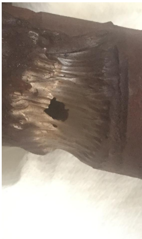
Figure 3: Severe internal erosion
