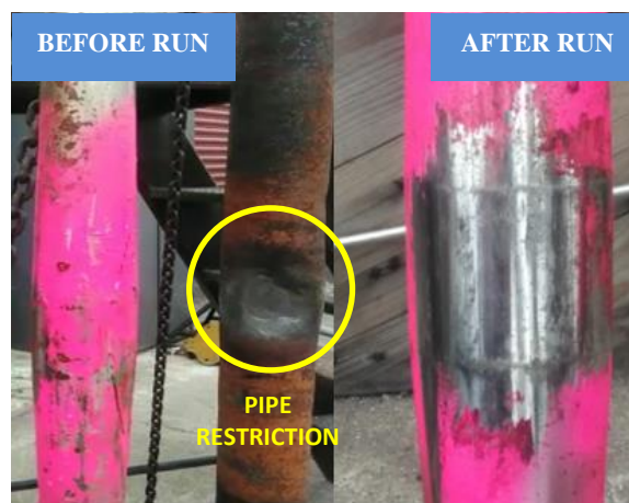
Figure 4: Casing restriction and swage before and after the run
