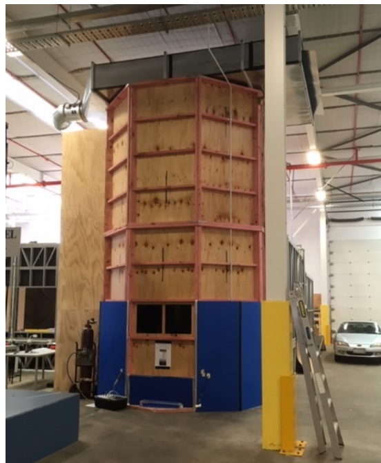
Fig. 2 Buoyancy Vortex Extension Cabinet, Wind-Tunnel Hall, University of Auckland.
