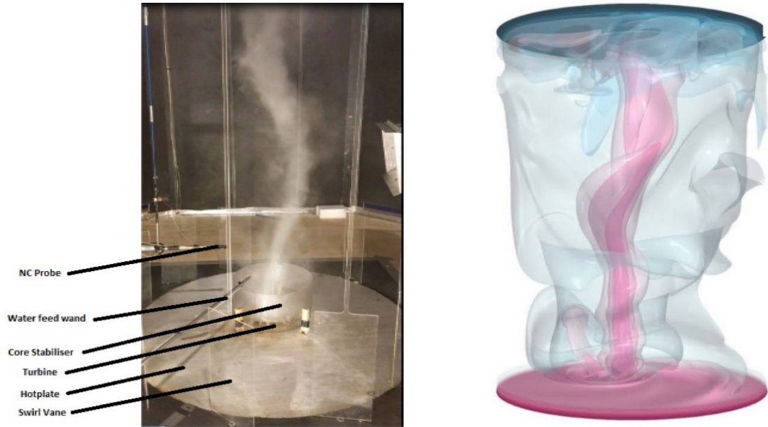
Fig. 3 Comparison of flow structures in our experiments and in the DNS of RRBC Experiment Ra \sim 109 , Ro \sim 1 , Fr \sim 0.5 : DNS Ra=108 , Ro=1 , Fr=0.5 (Horn and Aurnou, 2018).
