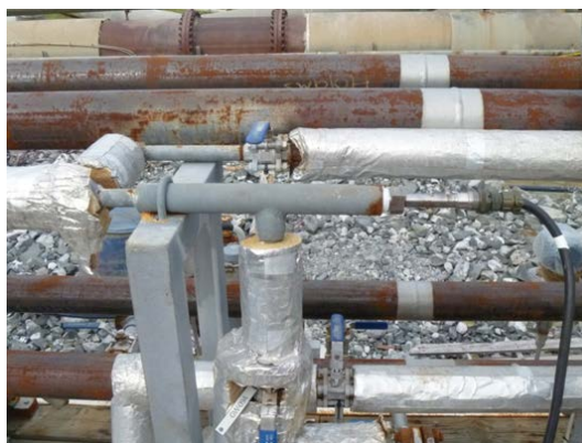
a) Small Bore Corrosion Test Loop ER Probe Access Point. (Note the discharge was implemented in a downwards orientation and the exit flow severely throttled by the control valve rather than the horizontal condition and longer exit pipe modelled.)
