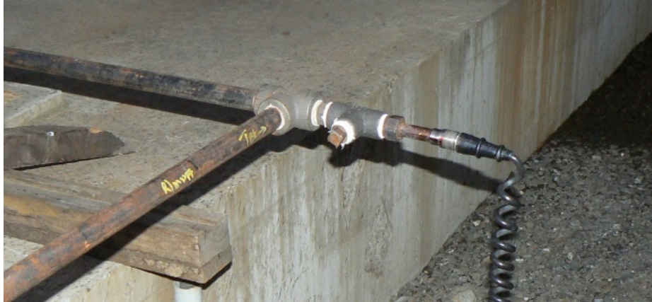
a) Typical 3/4 inch test T and ER probe arrangement.
