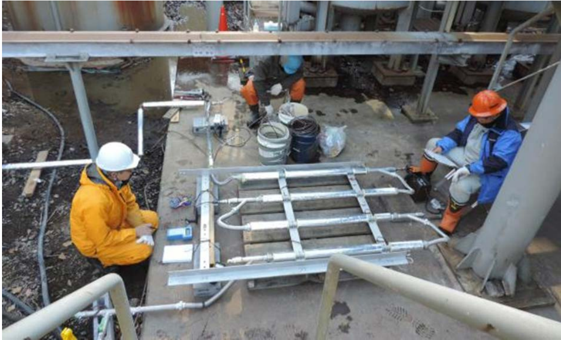
• Figure 5: Illustration of GERD corrosion test loop with Y arrangement being used for acidic brine testing, Osato et. al. (2016).
