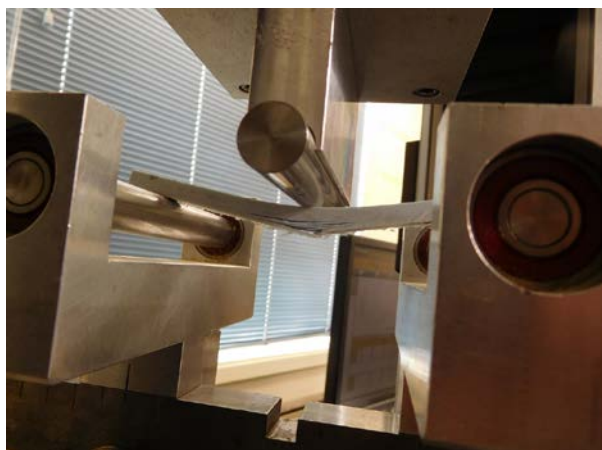
Figure A2: Flexural testing showing normal fracture mode of a well-performing FRP sample.
