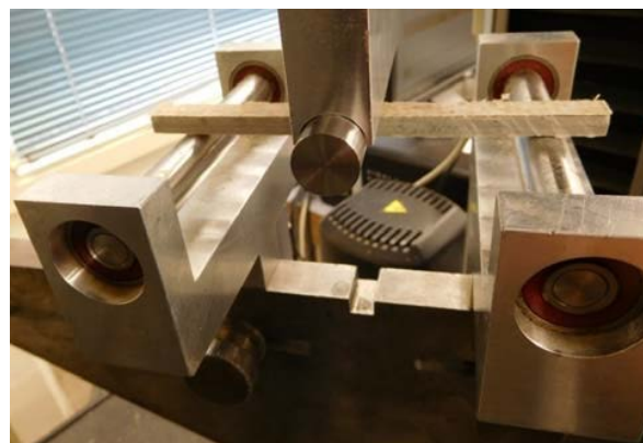
Figure A1: Flexural testing set-up.
