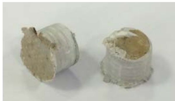
Figure 6: Photograph of intact, undamaged 16 mm cores, sampled below the Drift Eliminator level.
