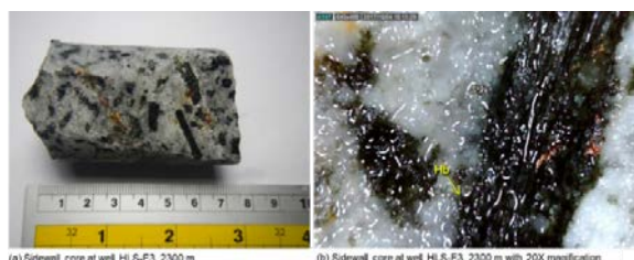
Figure 15. Sidewall core sample from drilling well at 2300 m showing granodiorite lithology (Nusantara, 2020).
