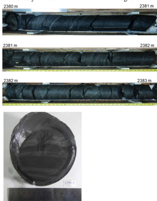
Figure 16. sidewall core from drilling well at 2300 m showing metasediment rock (Nusantara, 2020)
