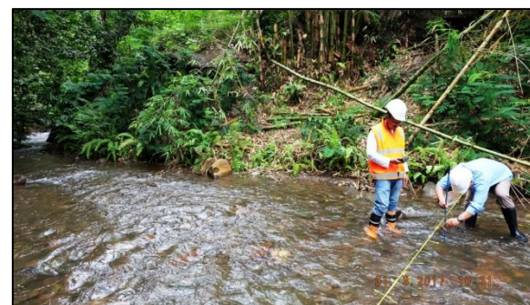
Figure 6. Flow rate measurement on one of the rivers. The flow rate is adequate but has a pH of 2.
