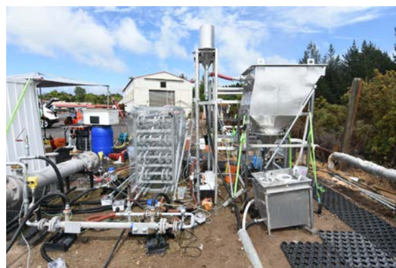
Figure 2: New pilot plant in operation including shell and tube and one double pipe HEX.
