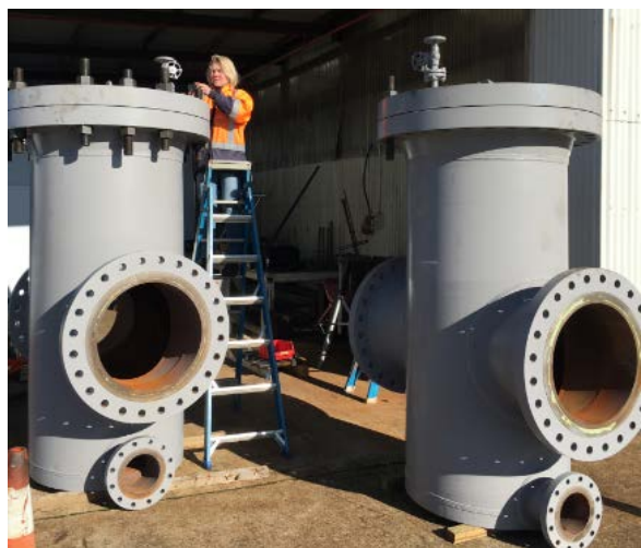
Figure 10 Example of a custom basket type strainer DN900 body, DN600 inlet
