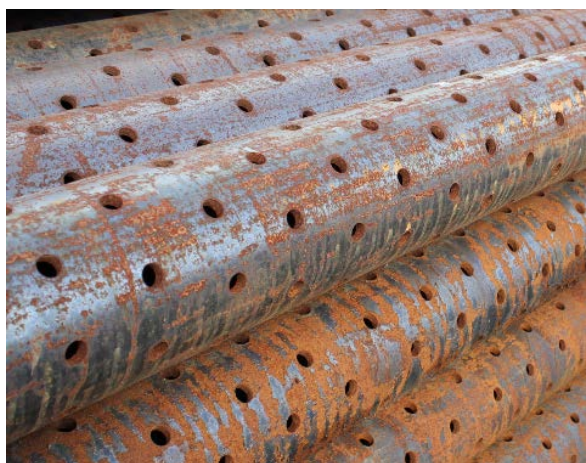
Figure 4 Well liner installed at the feed zone
