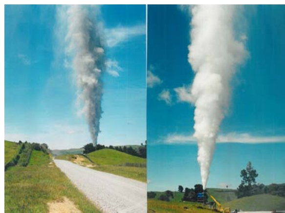
Figure 5 Vertical discharge of well with sand/slit/gravel (left) and without (right).
