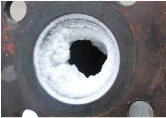
Figure 2 Scale deposition in pipe
