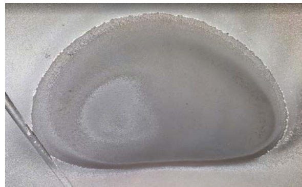
Figure 1: During internal inspections biased wear and erosion pattern was found where flow from the orifice plates impacted the downstream separator inlet manifold
