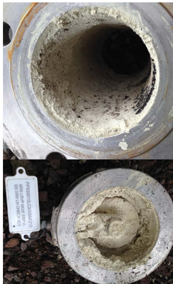
Figure 7: Sulphur deposits on LRVP moisture separator drain line (above) and check valve.
