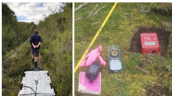
Figure 4: left: MALA GroundExplorer GPR 80MHz antenna; right: Tromino HVSR passive seismic device in use on site.
