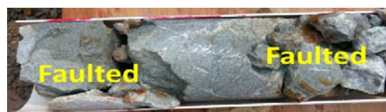
Figure 6: Core sample on faulted formation at particular depth of "DP" Well.
