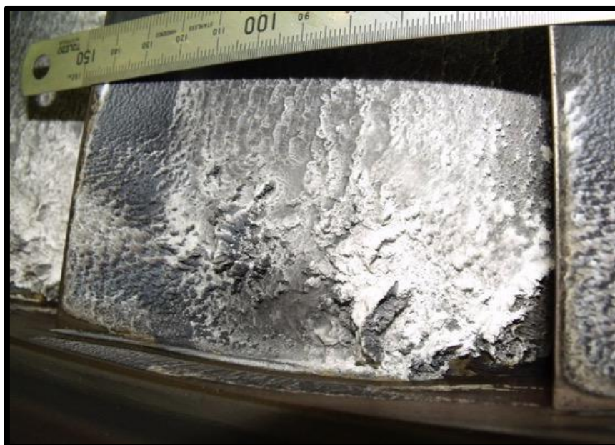
Figure 5: Example of Significant Geothermal Steam Turbine Deposits on a 1 st Stage Stationary Blade/Nozzle Due to Reheating of a Turbine Liquid Film and Suboptimal Steam Purity Conditions
