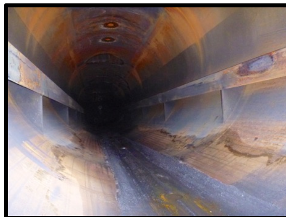
Figure 6: HEX 2 Tube Bundle Inspection – Late 2018 – HEX Shell Corrosion and Corrosion Products on Bottom
