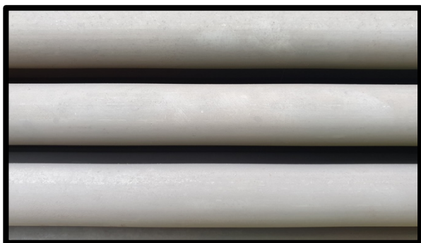
Figure 26: HEX1 Tubes with No Active Corrosion
