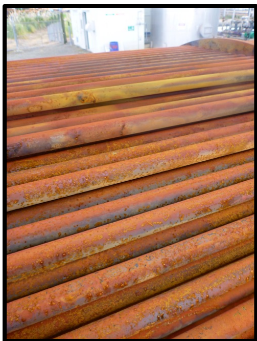
Figure 5: HEX 2 Tube Bundle Inspection – Late 2018 – Rusting and Pitting Present
