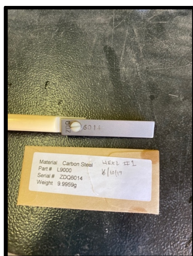
Figure 22: HEX1 Corrosion Coupon after 114 Days in Service Exposure with Sodium Hydroxide and Steamate PAS6074 Dosing
