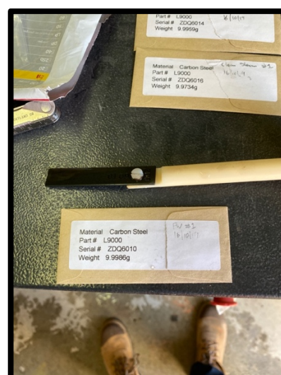
Figure 23: Feedwater Corrosion Coupon after 114 Days In Service Exposure with Sodium Hydroxide and Steamate PAS6074 Dosing
