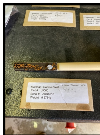
Figure 24: Clean Steam Corrosion Coupon after 114 Days in Service Exposure with Sodium Hydroxide and Steamate PAS6074 Dosing
