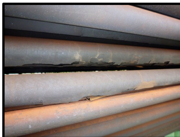
Figure 7: HEX 2 Tube Bundle Inspection – Late 2018 – Flaking Oxides
