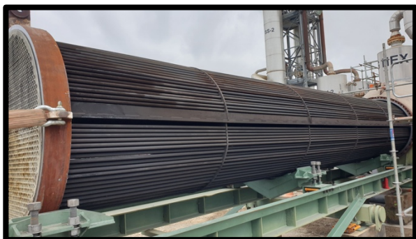
Figure 25: HEX1 Full Bundle with No Active Corrosion Present
