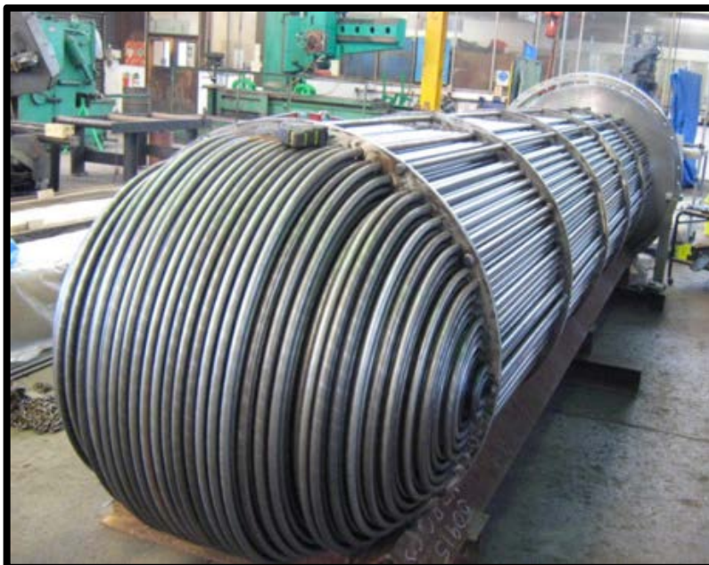
Figure 3: NTGA Carbon Steel Tube Bundle under Construction
