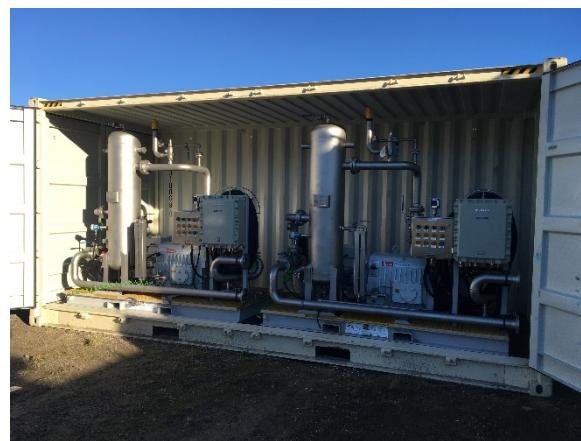
Figure 6: Pentane Evacuation Skids in storage at Ngatamariki
