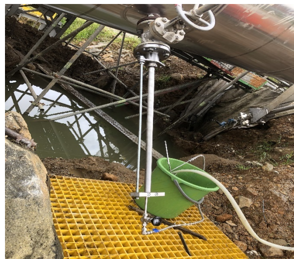
Figure 4: Traversing isokinetic probe with a 5.0 mm face ID nozzle, which is mounted onto the sampling port and connected to a stainless-steel cooling coil to collect steam condensate samples.
