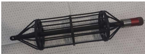
Figure 2: Typical Cage-Type Go-Devil
