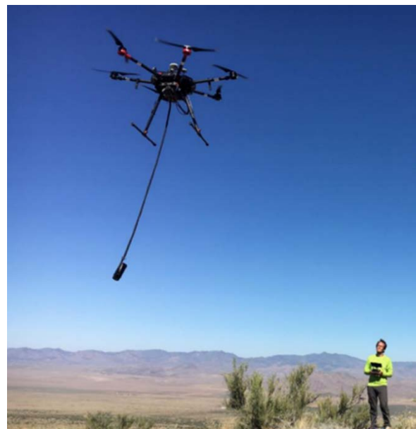
Figure 2: Image of the Matrice 600 drone used for the magnetic survey (Photo Credit: Global UAV: Pioneer Aerial Surveys Ltd).
