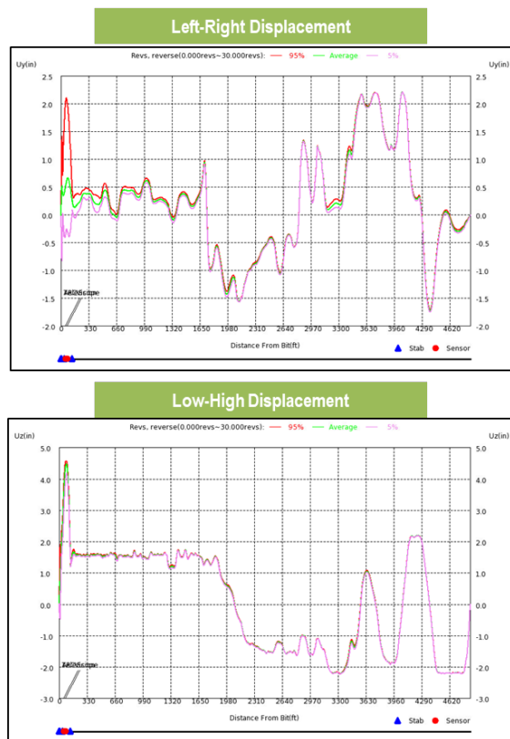
Figure 20. Casing left-right and low-high displacement.
