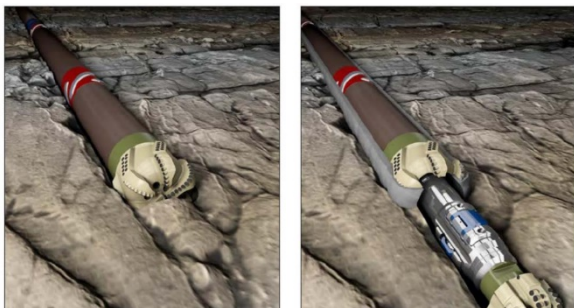
Figure 3. Casing drilling bit drill-out process.
