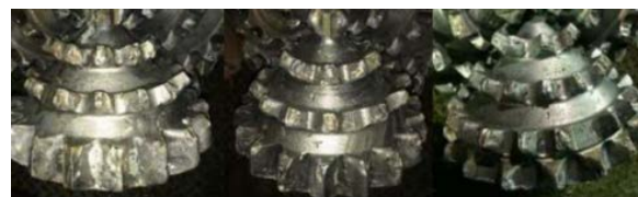
Figure 10. 12.25-in milled tooth bit condition after drill-out process.
