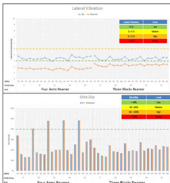
Figure 17. Vibration results from the dynamic simulation.
