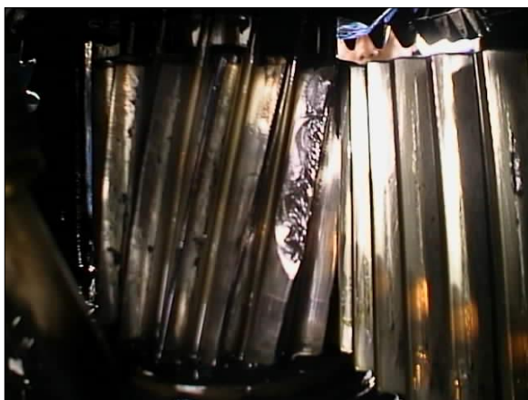
Figure 2: Severe gear tooth defect of CT gearbox
