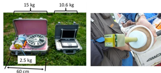
Figure 4: Picture of dewar vessel containing SQUID with receiver unit (left) and SQUID sensor (right).
