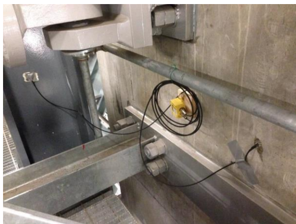
Figure 9: Thermocouple monitoring installation of Concrete and steel columns.
