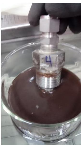
Figure 2: Bench top testing with a thermowell from the plant to inform solvent selection and cleaning design.
