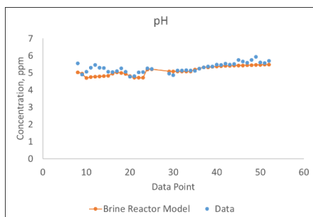
Figure 9: Model chemistry outputs from the Brine Reactor Model for pH.
