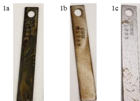
Figure 1. All coupons were exposed to the brine in Table 1, pH=7.4 for 5 minutes. 1a) No inhibitor - fail. 1b) Amino acid 1 - mixed. 1c) Amine 1 - pass.
