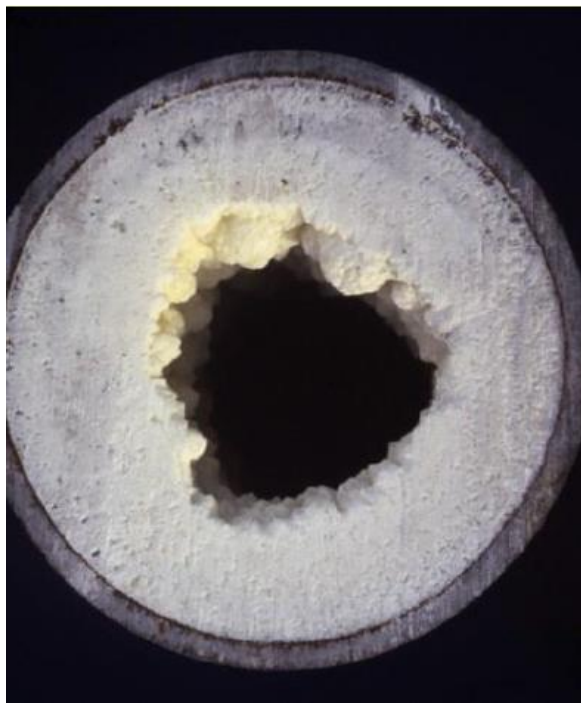
Figure 1. Calcium carbonate scale formation due to geothermal brine.
