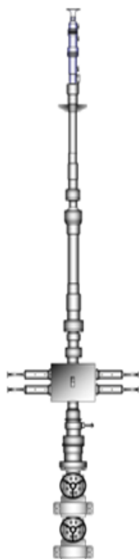
Figure 4: Schematic diagram of the Slickline HDFU Pressure Control Equipment (PCE) stack.
