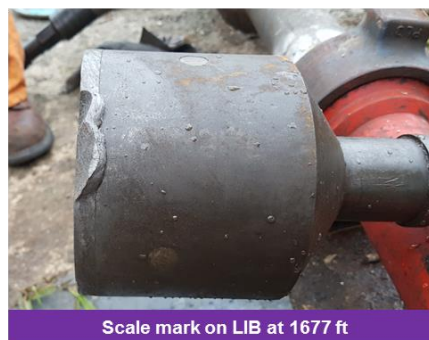
Figure 8: Recovered fish wire at the surface and IB mark at 1,677 ft.
